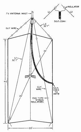
Where roof space is at a minimum, a pair of guy wires supporting a TV antenna installation can be used as the radiating portions of a 7-mc. (and 21-mc.) "inverted-V" transmitting antenna.
